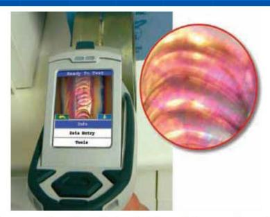
CCD camera and small-spot feature isolates and stores small sample area measurements.
