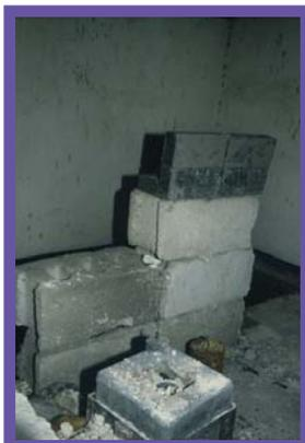
Figure 27: Improvised shield to test whether sources were leaking.
