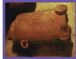
*Figure 32 (right): Old container with radioactive sources for industrial use.*
