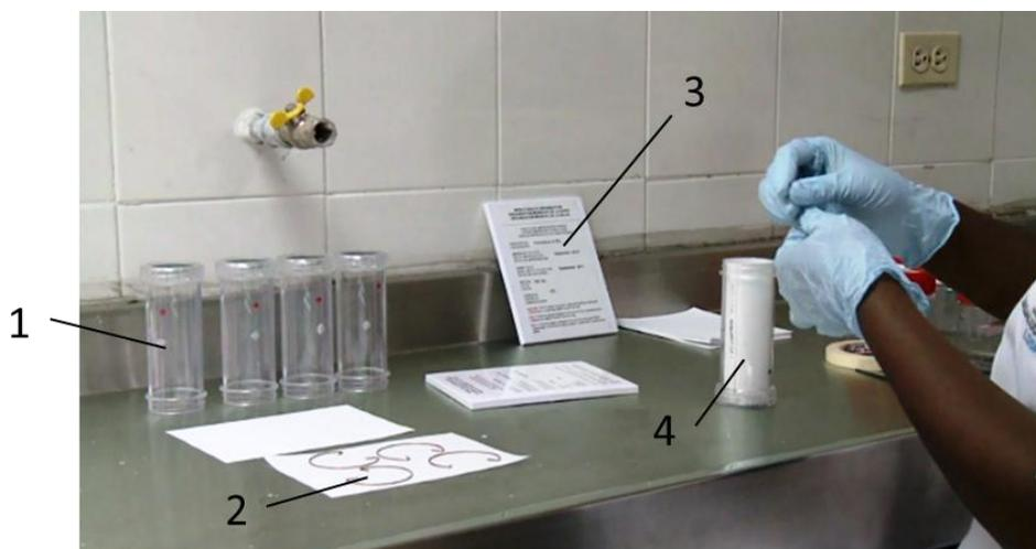
1. exposure tubes (red dot), 2. clips, 3. box with impregnated papers, 4. control tube (green dot)
