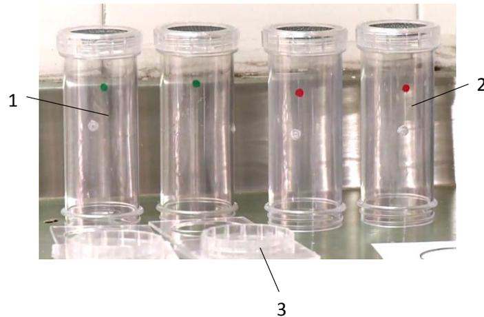
1. Control/holding tubes (green dot), 2. exposure tubes (red dot), 3. slide units
