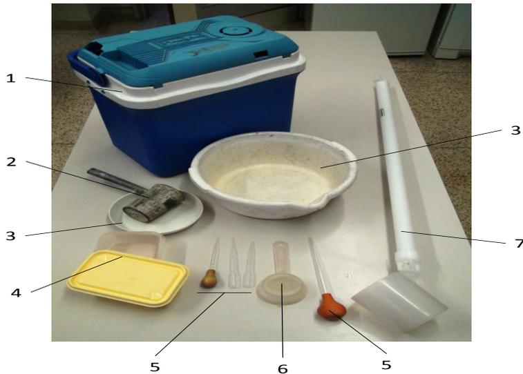
1. cool box, 2. ladle, 3. trays, 4. covered container, 5. pipettes, 6. strainer, 7. dipper.
