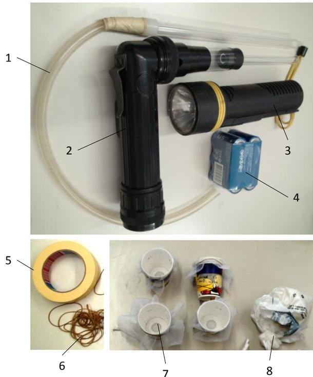
1. mouth aspirator, 2. mechanical aspirator, 3. flashlight, 4. spare batteries, 5. adhesive tape, 6. rubber bands, 7. paper-cups with netting, 8. cotton wool.
