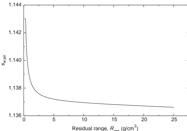
FIG. 21. Spencer–Attix ( $\Delta = 10$  keV) stopping-power ratios, water to air, for clinical proton beams as a function of the beam quality index  $R_{res}$ . The curve is a fit to monoenergetic stopping-power ratios calculated by Medin and Andreo using the Monte Carlo code PETRA [151, 152]. The data include the transport of secondary electrons and nuclear inelastic processes, and the basic proton stopping powers are taken from ICRU Report 49 [118].
