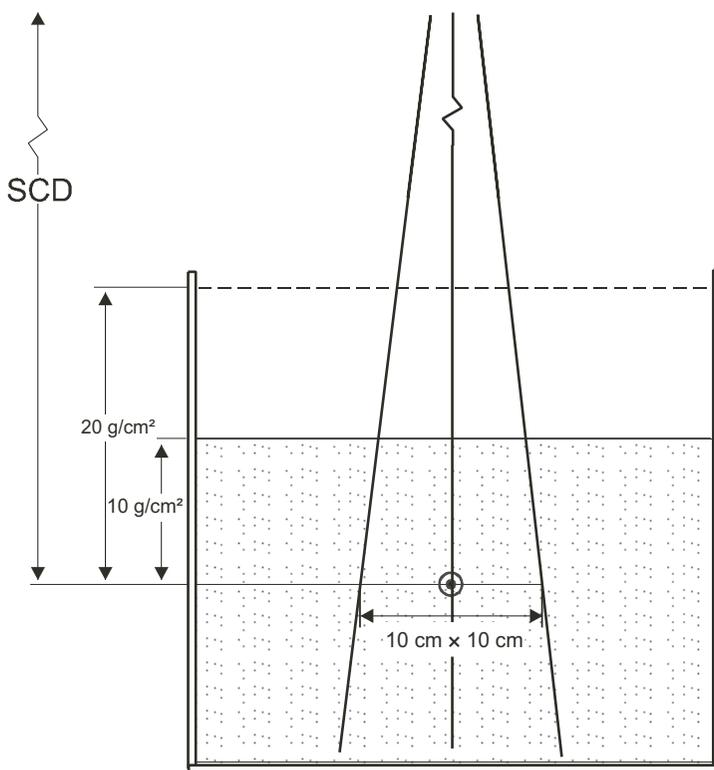
FIG. 6. Experimental set-up for the determination of the beam quality index  $Q$  ( $TPR_{20,10}$ ). The source-to-chamber distance (SCD) is kept constant at 100 cm and measurements are made with 10 g/cm<sup>2</sup> and 20 g/cm<sup>2</sup> of water over the chamber. The field size at the position of the reference point of the chamber is 10 cm x 10 cm. Either a cylindrical or a plane-parallel ionization chamber can be used.
