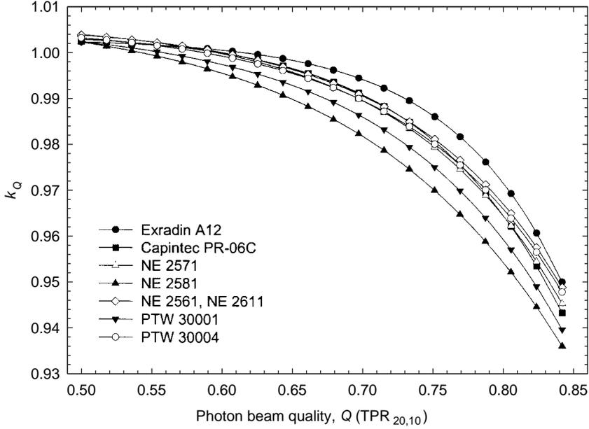
FIG. 7. Sigmoidal fits of calculated values of  $k_Q$  for various cylindrical ionization chambers commonly used for reference dosimetry, as a function of photon beam quality,  $Q$  ( $TPR_{20,10}$ ). Open symbols correspond to graphite walled ionization chambers, solid symbols to plastic walled chambers. Data from Table 14.
